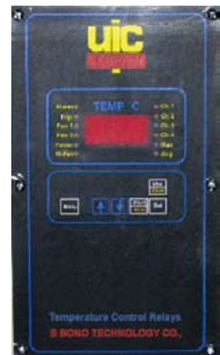
Temperature Indicator and Controller Power: 110/220V, 50/60Hz Contactor: AF Control, Alarm & Trip Temperature Range: 1°C~199°C Sensor: PT-100Ω x 3 Protocol(option): RS485/4~20mA
